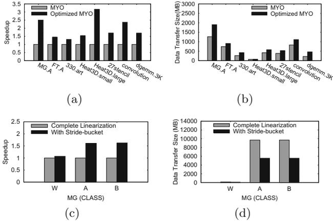
**Fig. 5.** Optimized MYO vs. MYO: (a) Execution time, (b) Total data transfer size; performance of complete linearization with and without stride-bucket optimization for varying input data sizes: (c) Execution time, (d) Total data transfer size
