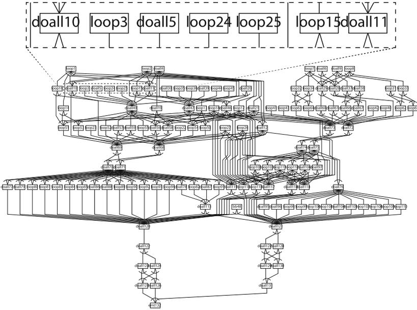
Fig. 3. Macro task graph after inline expansion
