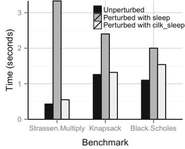
**Fig. 5.** The effect of perturbing existing computational kernels with simulated network dependencies. We sleep on a timer (either the OS thread or using `epoll` through the Cilk IO library) to simulate these network dependencies. Perturbations are random, and calibrated to happen for 50% of total *CPU* time.
