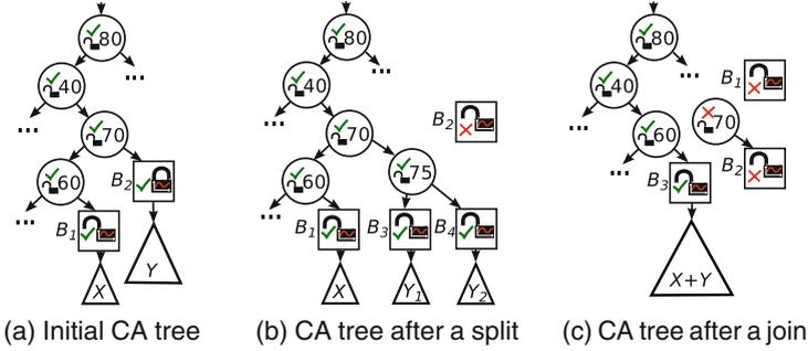
**Fig. 2.** Effect of the split and join operations on the CA tree of Fig. 2a.
