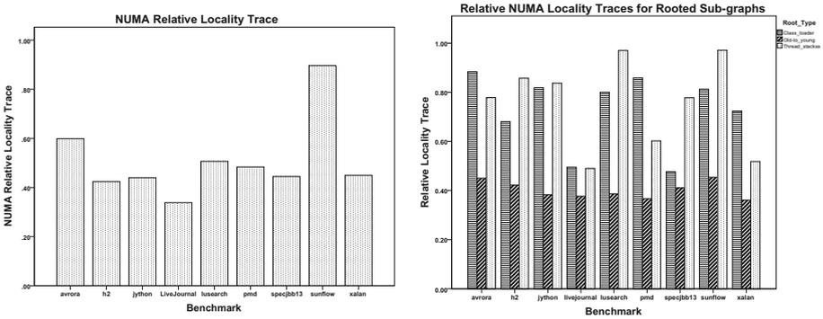
**Fig. 2.** (a) Relative NUMA Locality Traces for evaluated benchmarks. On average, 50 % of objects are local within rooted sub-graphs. (b) Relative NUMA Locality Traces for various root types: old-to-young, thread stacks, and class loader roots. An old-to-young rooted sub-graph exhibits relatively low locality.
