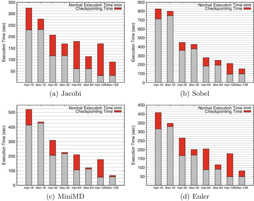
**Fig. 3.** Normal execution and checkpointing times of MPI and DISC implementations of four applications with varying number of nodes.
