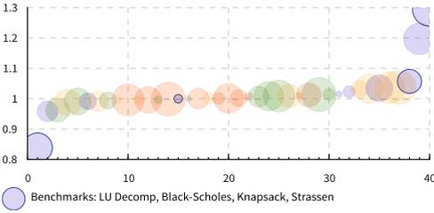
**Fig. 4.** The overhead of adding Concurrent Cilk to the Cilk scheduler. The Y axis is the speedup/slowdown factor (higher better), and the X axis is the count of benchmarks. Each color represents one of the benchmarks from the set of regression tests, and for each benchmark there is a different bubble for each thread setting, where larger bubbles imply more threads (Color figure online).
