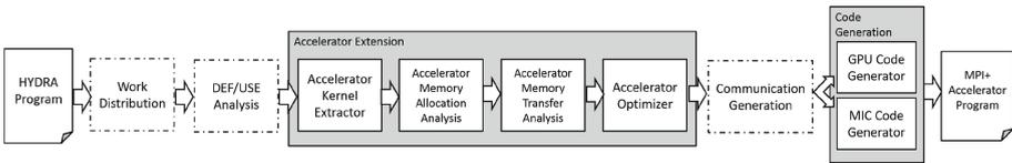
**Fig. 1.** HYDRA compiler translation process: grey boxes represent the new passes in the HYDRA compiler.
