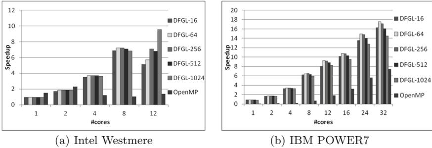
**Fig. 6.** Smith-Waterman using 2 sequences of 100k elements each. Results are for DFGL optimized code with loop tiling using tile sizes between 16 and 1024, and OpenMP baseline with parallelism obtained via loop skewing.
