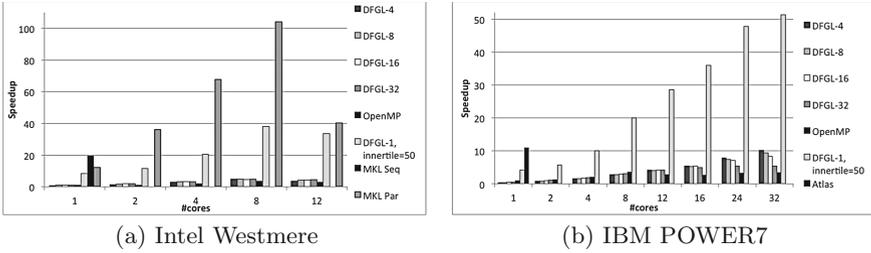
**Fig. 7.** Cholesky Factorization using  $2000 \times 2000$  matrix. Results are for loop tiling using tile sizes between 4 and 32, OpenMP parallelism, data tiling resulting of the inner steps and reference MKL/Atlas implementations.
