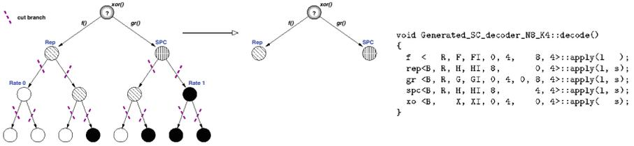
**Fig. 4.** Generation process on a small binary tree ( $N = 8$ ). The tree is cut and the computations are versioned according to the location of the frozen bit. The final code generated is in the right.
