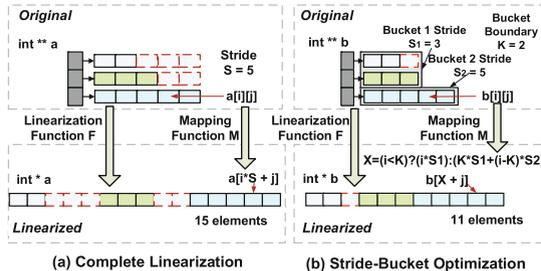
**Fig. 2.** Different linearization schemes for handling data transfers for dynamically allocated multi-dimensional arrays
