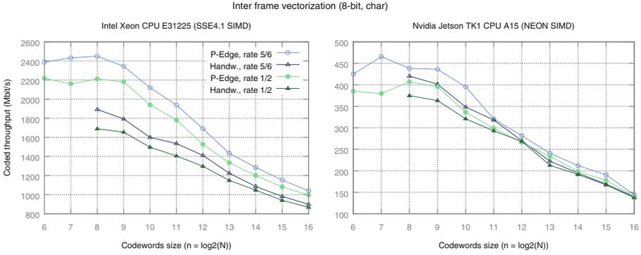
**Fig. 7.** Performance comparison between several code rates of 8-bit fixed point decoding stages (running on the Intel<sup>®</sup>Xeon<sup>®</sup>CPU E31225 and, respectively, on the Nvidia<sup>®</sup>Jetson TK1<sup>®</sup>CPU A15). Circles show P-EDGE results. Triangles show our former “handwritten” implementation [8].
