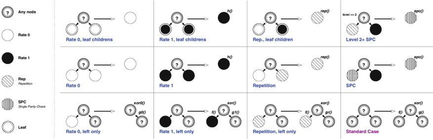
**Fig. 3.** Subtree rewriting rules for processing specialization.
