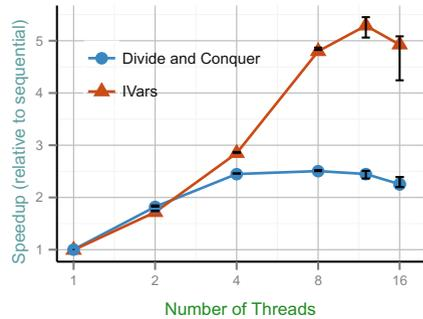
**Fig. 8.** A wavefront algorithm ran in two modes: first, in a divide-and-conquer recursive structure that divides the matrix into quadrants, executing the NW sequentially, and the NE and SW in parallel. The second mode is to simply fork a computation for each tile, and let IVars track the inter-tile data dependencies.
