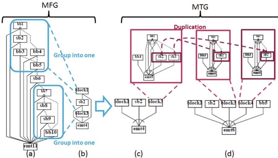
Fig. 5. Overview of the macro task fusion technique
