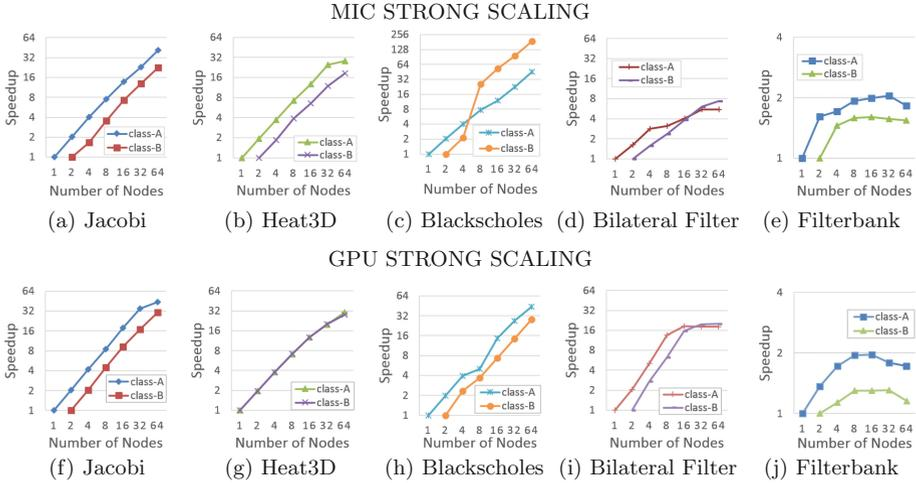
**Fig. 2.** Strong scaling experimental results of five benchmarks on MIC cluster(a-e) and GPU cluster (f-j). The speedup of the class-A problem is relative to a single-node performance. The speedup of class-B problem is relative to the performance of a configuration with the smallest number of accelerators that allow the program to be executed successfully.
