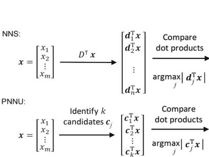
**Fig. 1.** A contrast between the naive exhaustive search and the NNU’s candidates approach in the number of dot-product computations. The  $k$  candidates are a subset of  $D$  which are selected by NNU. Increasing the  $\alpha$  and  $\beta$  parameters in NNU increases  $k$ , where  $k \leq \alpha \cdot \beta$ .
