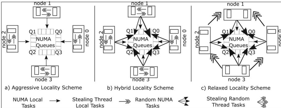
**Fig. 1.** Various topology-aware GC schemes. (a) aggressive scheme only processes local-node tasks (b) hybrid scheme distributes tasks across all nodes but steals from local node only. (c) relaxed scheme processes random tasks from any node
