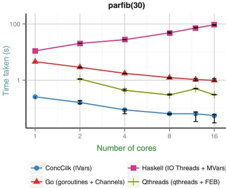
**Fig. 6.** A comparison of lightweight threaded runtimes with parallel fibonacci implemented by blocking on a **first-class synchronization object**. Concurrent Cilk does well, because of lazy thread creation. Each synchronization on an IVar *could* block, but not all do. Thus, initialization overhead is only incurred when needed.
