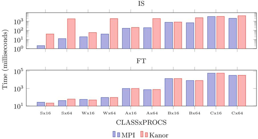
**Fig. 9.** Comparison of Kanor to MPI implementations of NAS Benchmarks Integer Sort (IS) and Fourier Transform (FT). NAS Benchmark class (S, W, A, B, C) denotes the size of the problem to be solved. Procs denote the number of processes used to solve the problem.
