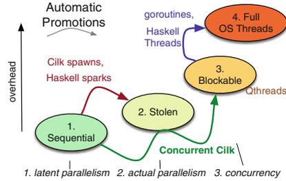
**Fig. 1.** State transitions possible for a fiber in each of several existing systems. At level (1), the fiber executes entirely within the stack of its caller. Work stealing transitions to (2) where a pre-existing system worker stack (allocated at startup) is used to execute the continuation of `f` in parallel. A blocked fiber requires additional storage for its state (3). Finally, blocking on underlying OS calls requires an OS thread (4).
