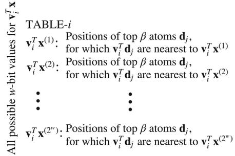
**Fig. 2.** Offline table preparation of content for TABLE- $i$  associated with the top principal component  $\mathbf{v}_i$  of  $\mathbf{D}$  for  $i = 1, 2, \dots, \alpha$ . For each possible  $w$ -bit value  $W$  for  $v_i^T \mathbf{x}$  the dictionary positions of the  $\beta$  atoms for which their scalar projections on  $\mathbf{v}_i$  are nearest to  $W$  are stored at table location  $W$ .
