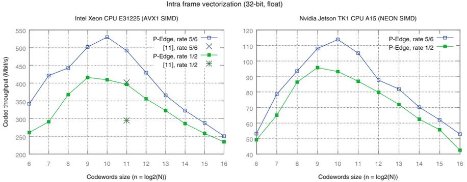
**Fig. 6.** Performance comparison between several code rates of 32-bit floating point decoding stages (running on the Intel<sup>®</sup> Xeon<sup>®</sup> CPU E31225 and, respectively, on the Nvidia<sup>®</sup> Jetson TK1<sup>®</sup> CPU A15).
