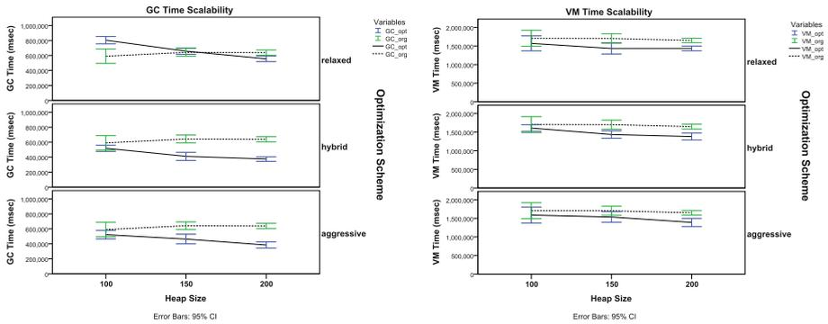
**Fig. 5.** GC (left) and VM (right) time scaling with heap size for Neo4j/LiveJournal. GC time decreases with heap size for our optimized versions, whereas the original implementation does not show any scaling.
