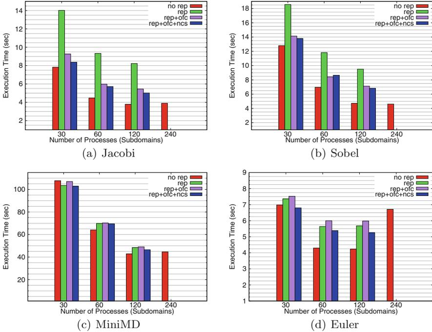
**Fig. 4.** Execution times of four applications without any replication (*no rep*), with plain replication (*rep*) and replication with improvements for cache utilization (*rep+ofc* and *rep+ofc+ncs*). Execution times for *no rep* with 1 process are 307.9, 398.9, 2686.2 and 213.2s in Jacobi, Sobel, MiniMD and Euler, respectively. The same execution times for the best replication version *rep+ofc+ncs* are 316.2, 474.5, 2738.3 and 214.8s.
