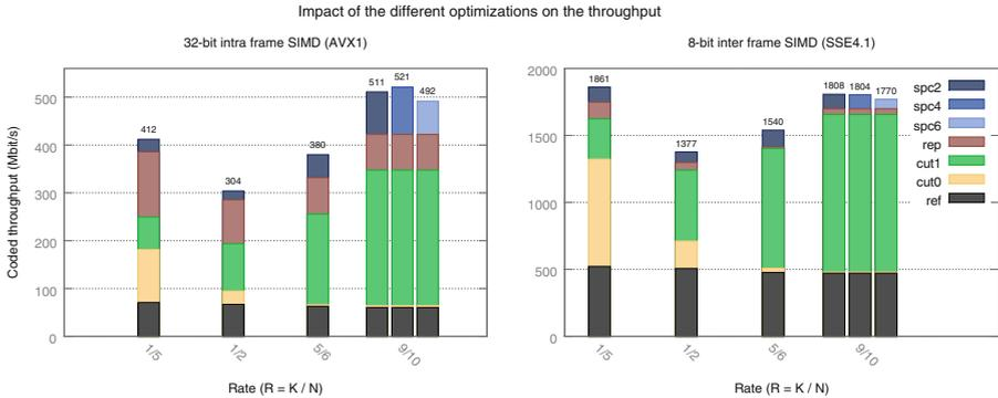
**Fig. 8.** Throughput depending on the different optimizations for  $N = 2048$ , for intra-frame vectorization on the left and intra-frame vectorization on the right, resp. (on the Intel<sup>®</sup>Xeon<sup>®</sup>CPU E31225).
