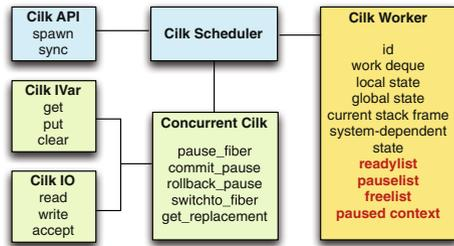
**Fig. 2.** The architecture of the modified Concurrent Cilk runtime system. Also pictured is the included, but optional, Cilk IO library. The bold red entries in the worker structure represent Concurrent Cilk extensions (Color figure online).
