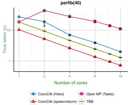
**Fig. 7.** Restricted task-only libraries’ performance on parallel fibonacci, with Concurrent Cilk (IVars) included for comparison. The IVar-based version does quite well here in spite of blocking threads on reads—it scales as well as TBB and raw Cilk (spawn/return), and outperforms Open MP.
