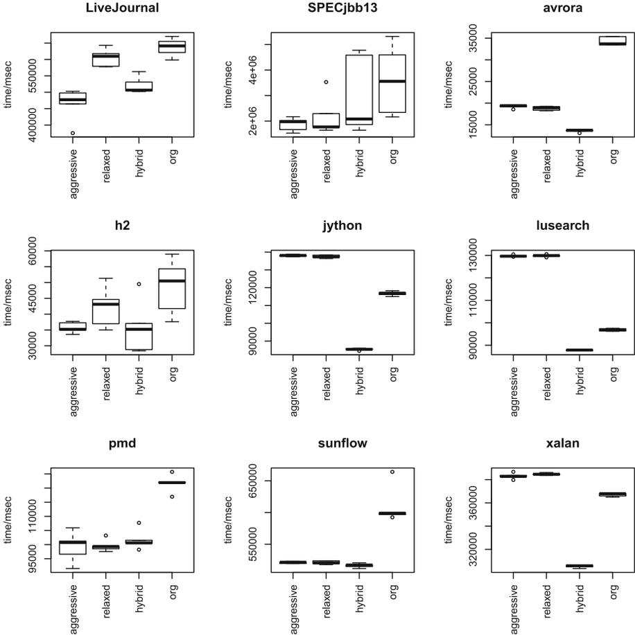
**Fig. 3.** GC time (i.e. pause time) for our three schemes. For small heaps (e.g. DaCapo programs), hybrid scheme gives the best results, whereas aggressive scheme is more effective for apps with larger heaps. (The default JVM is labeled *Org*.)
